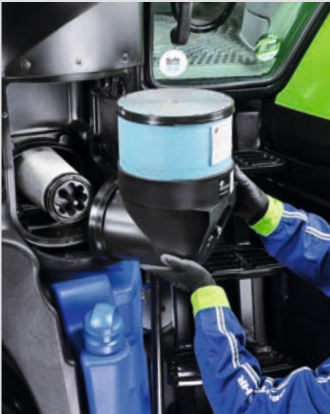
↑ The engine air filter is easy to insert and remove.
