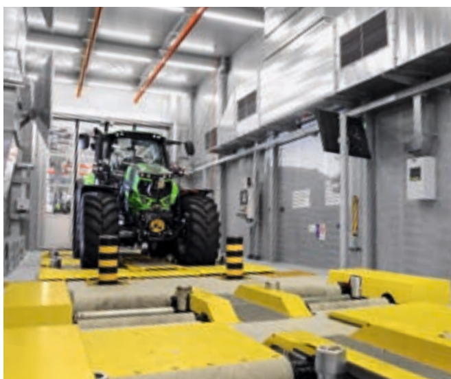
⬆ Unique in tractor manufacturing: chassis dynamometer and axle suspension test bed.
