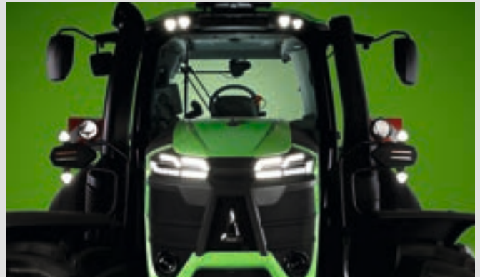
↑ LED package with up to 40,000 lm.
