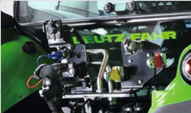
↑ The compressed air brake system decelerates trailers in all weight categories reliably and safely.
