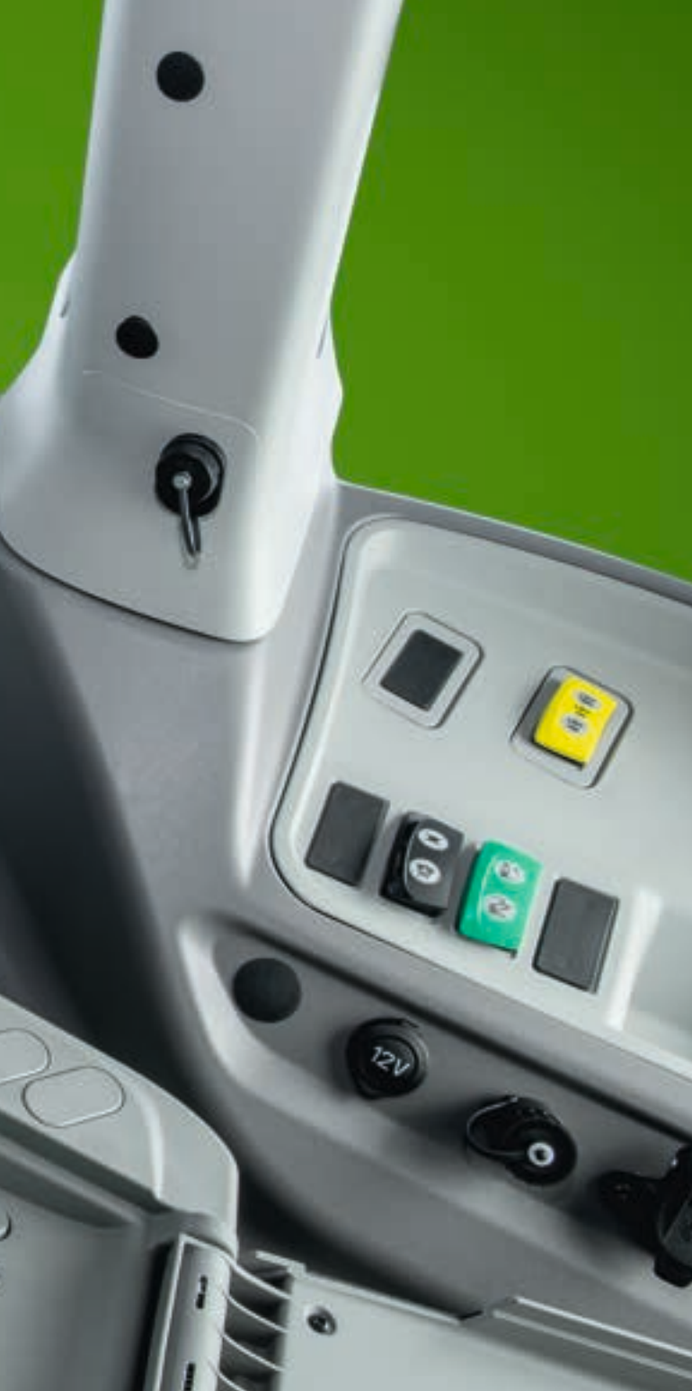
↑ The cross-control lever with rocker switch controls three hydraulic control valves.
